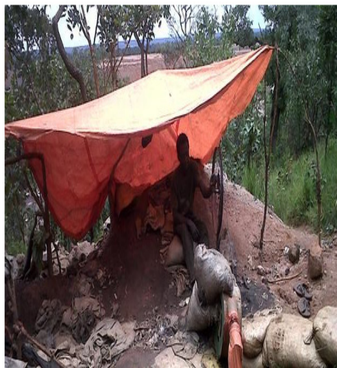
Improvised ventilation for a mine shaft at the Tilwezembe site, near Kolwezi, Katanga
